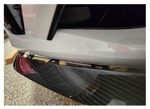
Note: In the spaces between where the new lip slides in, some non-Blackwing cars have small tabs which prevented the lip from siting properly. Either remove the tabs from the bumper with a knife, or Dremel out a slot in the new lip to slide over these bumps.
