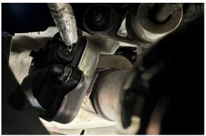
10. Unplug the wiring harness from the exhaust valve actuators located on the inner most driver and passenger tip pipes. To release the plug, slide the white locking clip away from the actuator, press down on the clip and slide the plug away from the actuator.
