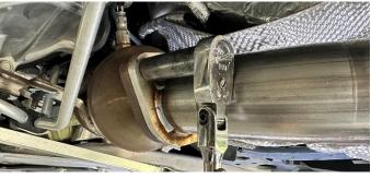
Secure the head pipe with the factory mounting nuts at the passenger side head pipe flange connection using a ratchet and 15mm deep socket, until the head pipe is snugly held in place. Leave the flange connection loose enough for adjustment.
