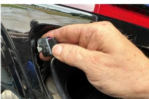
Both the driver and passenger side valve wiring harness connections should now be disconnected and hanging clear of the stock rear mufflers.
