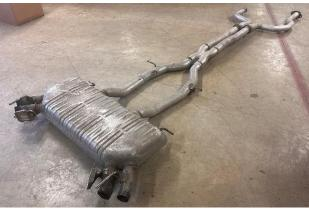
16. Slide the entire stock exhaust assembly rearward until the stock flange and sleeve clamp are free from the exhaust catalyst pipes. Lower the front of the exhaust, then slide it forwards to allow the rear muffler, valve actuators, and rear muffler hangers to move forward and down to clear the rear fascia while CAREFULLY removing the exhaust from the vehicle.
