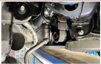
Slide the axle pipe hanger into the corresponding grommet as shown.
