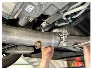
10. Locate the driver side axle pipe assembly and a 3.0" clamp. Repeat INSTALL STEPS 7-9 on the driver side of the vehicle.
