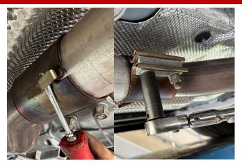
6. Use a flat head screwdriver to pry open the locking tab on the driver sleeve clamp, located just aft of the driver side exhaust catalyst. Next, use a 3/8" drive ratchet and 15mm deep socket to loosen both nuts on the sleeve clamp as shown.
