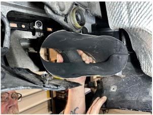
**20. CAREFULLY** remove the driver side OEM Bezel Tip from the rear fascia as shown.
