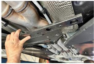
5. Move the plastic underside panels down and slide the center Cross Member out from above the paneling, to allow the Cross Member to be removed from the vehicle.
