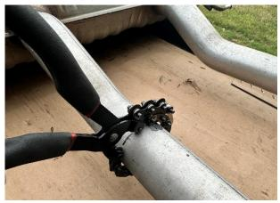
**28.** Using a chain cutter or similar device, cut both the driver and passenger side exhaust pipes at the marked locations.
