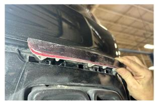
17. CAREFULLY remove the two reflectors on each side of the vehicle to enable access to the four rivets (2 per side) securing the top of the OEM Bezel Tips to the rear fascia. Each Reflector is snapped in place using two tabs, which can be pushed out from inside the fascia.
