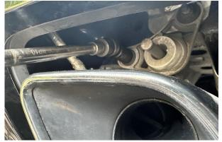
**NOTE:** An additional helper (or two) is highly recommended for **REMOVAL STEPS 12-13**. The rear fascia must be pulled away from the exhaust for the valve actuators to clear during exhaust removal.
