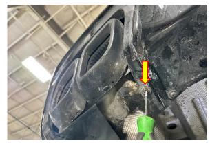
19. Remove the screw securing the lower inside position of the driver side OEM Bezel Tip to the rear fascia using a T15 Torx Screwdriver. Note that this screw will not be reused.
