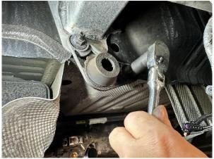
21. Use a 3/8" drive ratchet and 15mm socket to remove both nuts securing each of the driver and passenger side rear hanger grommet assemblies. Set aside the fasteners in a protected location to be reused during the full cat back exhaust installation (INS5396).
