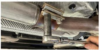
3. Locate the driver side head pipe. Fully insert the head pipe into the factory driver sleeve clamp as shown. Secure the head pipe with the sleeve clamp nuts using a ratchet and 15mm deep socket, until the head pipe is snugly held in place. Leave the clamp connection loose enough for adjustment.
