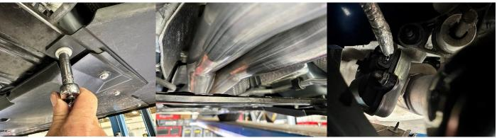
15. Locate the cross member and all fasteners set aside in REMOVAL STEPS 1-2 (CT4-V BW ONLY) or REMOVAL STEPS 3-5 (CT5-V BW/NON-BW ONLY) of the stock exhaust removal process. Reinstall the cross member and plastic underside paneling. Installation is reverse of removal. Installation Complete. This concludes the installation of your CORSA Performance exhaust system.
