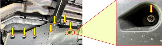
1. To access the center Cross Member, remove the 14 bolts (7 per side) securing the plastic underside panels over the ends of the Cross Member with a 3/8" drive ratchet and 10mm socket. Note that two of the fasteners (1 per side) are in a recessed pocket, and two more of the fasteners (1 per side) secure the oil cooler lines along with the underside paneling.
