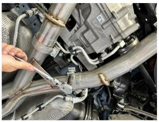
11. Secure both axle pipes using a ratchet and 15mm deep socket, until the axle pipes are snug on both X-Pipe outlet ends. Leave the clamp connections loose enough for adjustment.
