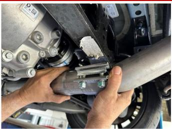
12. Align the outlet ends of both axle pipes with both inlets of the FACTORY REAR MUFFLER section. Move the muffler section forward until the pipes are touching against both axle pipes, then position both sleeve clamps to center on the split between the pipes as shown.
