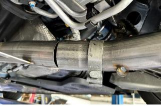
9. Slide the passenger axle pipe assembly onto the passenger x-pipe outlet, with a recommended pipe overlap of 1.75 inches. Rotate the axle pipe until the hanger is horizontal as it runs through the stock grommet.
