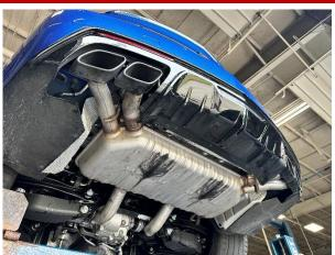
30. Reinstall the FACTORY REAR MUFFLER exhaust section into the vehicle. Installation is the reverse of REMOVAL STEPS 9-13 (CT4/5-V Blackwing) or REMOVAL STEPS 9, 14-16 (CT5-V Non-Blackwing)
