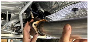
Locate the passenger side head pipe assembly and the two nuts set aside during REMOVAL STEP 7. Slide the flange onto the studs from the passenger side catalyst as shown.
