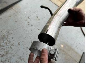
Locate the passenger side axle pipe assembly and a 3.0" clamp. Slide a clamp over the inlet of the passenger axle pipe, so that the nut will be located on the inside of the axle pipe and facing downwards.
