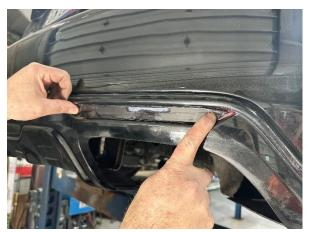
**25. CAREFULLY** align and reinstall the two reflectors on each side of the vehicle by snapping the two mounting tabs in place.
