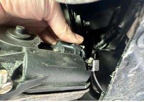
**NOTE:** An additional helper (or two) is highly recommended for **REMOVAL STEPS 15-16**. The rear fascia must be pulled away from the exhaust for the valve actuators to clear during exhaust removal.
