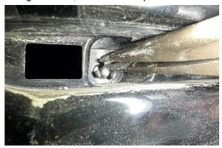
18. Use a pair of needle nose pliers to twist off and remove the three metal ears on each of the two driver side rivets. Next, use a punch to push the center of each rivet through the mounting holes in the rear fascia to remove the rivets.
