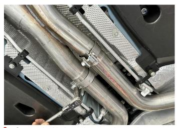
6. Secure the X-pipe using a ratchet and 15mm deep socket, until the X-Pipe is snug on both head pipe outlet ends. Make sure the clamp nuts and studs are vertical while snugging the clamps. Place a jack stand or similar device under the rear of the X-Pipe for support. Leave the clamp connections loose enough for adjustment.
