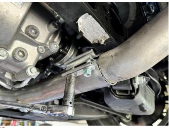
13. Secure the FACTORY REAR MUFFLER section with both sets of sleeve clamp nuts using a ratchet and 15mm deep socket, until the muffler section is snugly held in place. Leave the clamp connections loose enough for adjustment.
