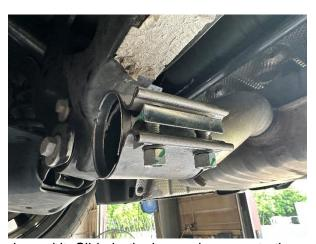
31. Locate the two supplied sleeve clamps from the hardware kit. Slide both sleeve clamps onto the cut location of the FACTORY REAR MUFFLER, with the nuts on the sleeve clamps facing towards the center of the vehicle as shown. Slide the sleeve clamps onto the pipes as far as possible; this will allow room for the installation of the CORSA double X-pipe tunnel section.
