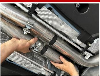
5. Position the X-Pipe so the cross brace located at the rear of the X-Pipe is facing CORSA logo side down and parallel with the ground, and the Xpipe outlets are centered around the rear differential. Slide each of the X-pipe inlet legs onto the two head pipe outlets ends, with a recommended pipe overlap of 1.75 inches.
