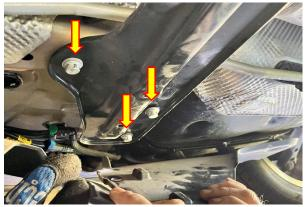
2. Remove the 6 bolts (3 per side) securing the Cross Member to the chassis using a 3/8" drive ratchet and 13mm socket, then move the plastic underside panels down and slide the center Cross Member out from above the paneling, to allow the Cross Member to be removed from the vehicle.
