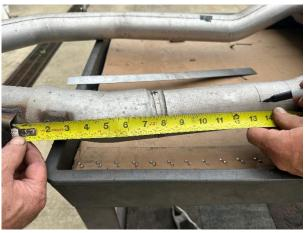
27. Measure 13.5" rearwards (towards the factory muffler) from the rearward edge of the driver side axle pipe hanger bracket as shown, following the outside profile of the exhaust pipe, to mark the CUT LINE.
