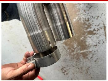
4. Locate the double X-pipe assembly and two 3.0" clamps. Slide a clamp over the inlet of each of the front legs of the X-pipe, so that the nuts will be located on the outside of the X-pipe and facing downwards.
