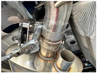
17. Secure the passenger inner tip pipe using a ratchet and 15mm deep socket, until the inner tip pipe inlet is snug on the muffler outlet. Leave the clamp connection loose enough for adjustment.
