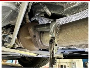
Remove both nuts at the passenger side flange connection, located just behind the passenger side exhaust catalyst, using a 3/8" drive ratchet and 15mm deep socket.
