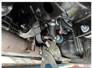
8. Remove the driver and passenger side axle pipe hangers (located in front of the rear suspension) from the factory grommets using grommet pullers or a similar device.
