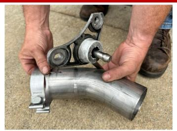
14. Locate a 3.0" clamp and the passenger inner tip pipe assembly. Slide the clamp over the inlet of the inner tip pipe, so that the nut will be located on the inside of the tip pipe inlet and facing downwards. Install the rear exhaust grommet onto the rear hanger position with the flat facing upwards as shown.
