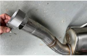
**6.** Locate a 2.75" clamp. Slide the clamp over the inlet of the passenger muffler assembly, so that the nut will be located on the inside of the muffler inlet and facing downwards.
