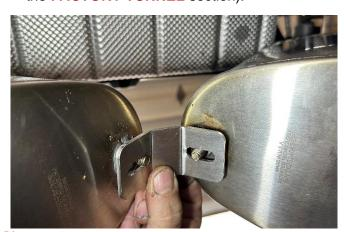
**41.** Locate the supplied 5/16" nuts and muffler tie bracket from the hardware kit. Slide the muffler tie bracket over the studs from both mufflers as shown.
