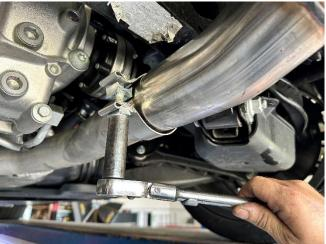
**39.** Rotate the passenger muffler upwards until the front muffler hanger is horizontal as it runs through the stock grommet, then secure the passenger muffler using a ratchet and 15mm deep socket, until the muffler inlet pipe is snug on the axle pipe outlet. Leave the clamp connection loose enough for adjustment.
