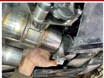
**38.** Rotate the passenger muffler upwards until the passenger inner tip pipe assembly slides onto the passenger muffler outlet, with a recommended pipe overlap of 1.625 inches.
