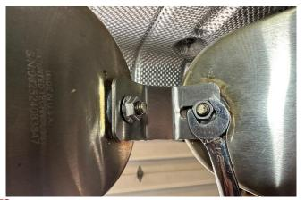
**42.** Secure the muffler tie bracket using a ½" wrench. Leave the nuts loose enough for adjustment.
