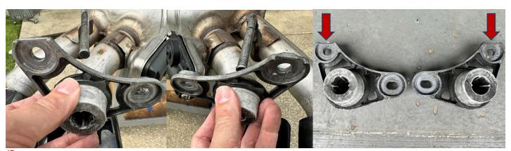
13. Remove both rear exhaust grommets from the exhaust hangers on the FACTORY REAR MUFFLER using grommet pullers or a similar device. Note the orientation of the grommets for the following installation step.
