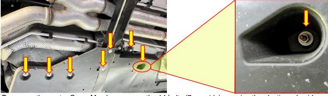
1. To access the center Cross Member, remove the 14 bolts (7 per side) securing the plastic underside panels over the ends of the Cross Member with a 3/8" drive ratchet and 10mm socket. Note that two of the fasteners (1 per side) are in a recessed pocket, and two more of the fasteners (1 per side) secure the oil cooler lines along with the underside paneling.
