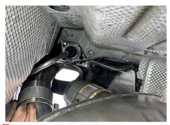
**37.** Rotate the passenger muffler as necessary to create clearance to install the passenger inner tip pipe hanger. Slide the inner tip pipe hanger into the corresponding grommet as shown.
