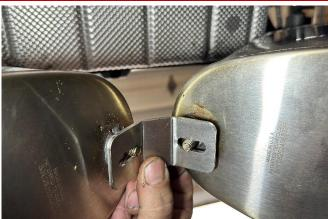
11. Locate the supplied 5/16" nuts and muffler tie bracket from the hardware kit. Slide the muffler tie bracket over the studs from both mufflers as shown.
