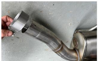
**32.** Locate a 2.75" clamp. Slide the clamp over the inlet of the passenger muffler assembly, so that the nut will be located on the inside of the muffler inlet and facing downwards.
