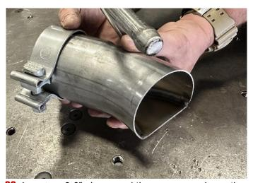
36. Locate a 3.0" clamp and the passenger inner tip pipe assembly. Slide the clamp over the inlet of the inner tip pipe, so that the nut will be located on the inside of the tip pipe inlet and facing downwards.
