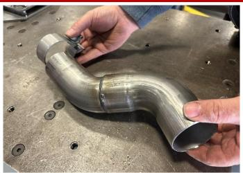
43. Locate a 2.25" clamp and the passenger outer tip pipe assembly. Slide the clamp over the inlet of the inner tip pipe, so that the nut will be located on the outside of the tip pipe inlet and facing downwards.
