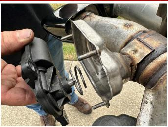
On the FACTORY REAR MUFFLER section, remove the three nuts on each valve actuator using a 1/4" drive ratchet and 10mm socket. Remove both FACTORY VALVE ACTUATORS from the valve assemblies on the muffler.
