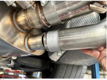
**24.** Slide the passenger outer tip pipe assembly onto the passenger muffler outlet, with a recommended pipe overlap of 1.625 inches.
