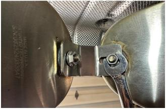
**12.** Secure the muffler tie bracket using a ½" wrench. Leave the nuts loose enough for adjustment.
