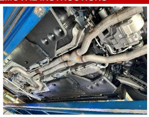
**30.** Reinstall the **FACTORY TUNNEL** exhaust section into the vehicle. Installation is the reverse of **REMOVAL STEPS 6-8**.
