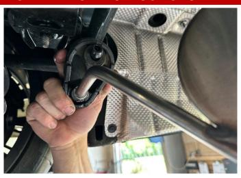
**34.** Slide the front muffler hanger into the corresponding grommet as shown.
