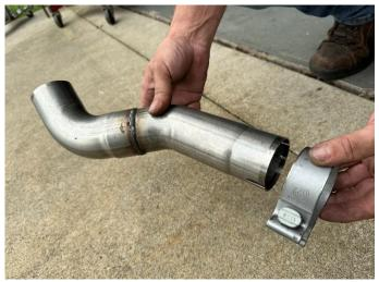
23. Locate a 2.25" clamp and the passenger outer tip pipe assembly. Slide the clamp over the inlet of the inner tip pipe, so that the nut will be located on the outside of the tip pipe inlet and facing downwards.
