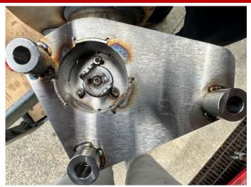
Locate the passenger muffler assembly and three of the supplied M6 bolts from the hardware kit. Rotate the valve actuator bracket on the CORSA muffler until the valve plate is in the fully open position as shown.
