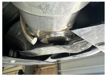
45. Rotate the passenger inner tip pipe until the flat on the bottom of the inner tip pipe and the inside lower edge of the factory bezel tip are parallel as shown.
