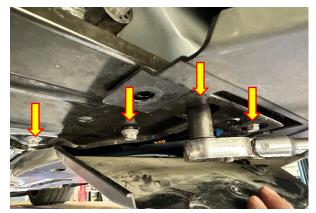
**4.** Remove the 8 bolts (4 per side) securing the Cross Member to the chassis using a 3/8" drive ratchet and 13mm socket.
