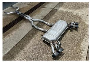
13. Push up slightly on the exhaust tip pipes, then slide the rear hanger grommet assemblies rearward to free them from the studs in the chassis. Next, slide the entire stock exhaust assembly rearward until the stock flange and sleeve clamp are free from the exhaust catalyst pipes. Lower the front of the exhaust, then slide it forwards to allow the rear muffler, tips, and valve actuators to move forward and down to clear the rear fascia while CAREFULLY removing the exhaust from the vehicle.
