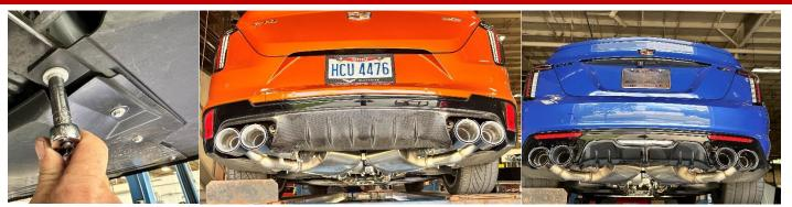
53. Locate the cross member and all fasteners set aside in REMOVAL STEPS 1-2 (CT4-V BW ONLY) or REMOVAL STEPS 3-5 (CT5-V BW/NON-BW ONLY) of the stock exhaust removal process. Reinstall the cross member and plastic underside paneling. Installation is reverse of removal. Installation Complete. This concludes the installation of your CORSA Performance exhaust system.
