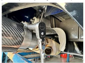
21. Adjust the rotation of the CORSA inner tip assembly until the CORSA logo is centered on the top of the tip, then secure the exhaust clamp at the tip inlet using a 15mm socket and 3/8" ratchet, until the tip is snug on the inner tip pipe. Leave the clamp connection loose enough for adjustment.
