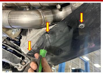
**48.** Locate the six screws set aside in **REMOVAL STEP 14.** Reinstall the 6 screws (3 per side) securing the side under paneling to the exhaust heat shielding using a T15 Torx Screwdriver.
