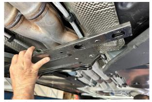
Move the plastic underside panels down and slide the center Cross Member out from above the paneling, to allow the Cross Member to be removed from the vehicle.
