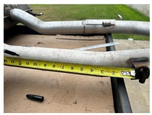
**26.** On the factory exhaust, measure 12" rearwards (towards the factory muffler) from the rearward edge of the passenger side axle pipe hanger bracket as shown, following the outside profile of the exhaust pipe, to mark the **CUT LINE**.
