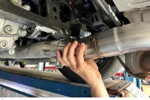
Slide the passenger muffler assembly onto the passenger axle pipe outlet (or passenger outlet of the FACTORY TUNNEL section), with a recommended pipe overlap of 1.75 inches.
