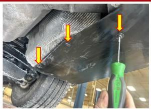
14. Remove the 6 screws (3 per side) securing the Side under paneling to the exhaust heat shielding using a T15 Torx Screwdriver.
