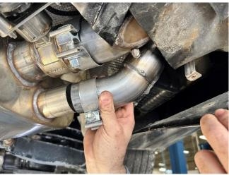
**44.** Slide the passenger outer tip pipe assembly onto the passenger muffler outlet, with a recommended pipe overlap of 1.625 inches.
