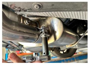
**25.** Secure the passenger outer tip pipe using a ratchet and 15mm deep socket, until the outer tip pipe inlet is snug on the muffler outlet. Leave the clamp connection loose enough for adjustment.
