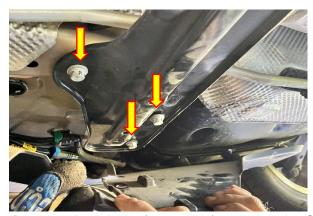
2. Remove the 6 bolts (3 per side) securing the Cross Member to the chassis using a 3/8" drive ratchet and 13mm socket, then move the plastic underside panels down and slide the center Cross Member out from above the paneling, to allow the Cross Member to be removed from the vehicle.
