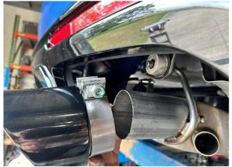
20. Locate a 3.0" clamp and one of the CORSA stainless (or Carbon) inner tip assemblies. Slide the clamp over the tip inlet, so that the nut will be located on top of the tip inlet and facing outwards. Slide the inner tip assembly onto the passenger inner tip pipe with approximately 1.75" of overlap.
