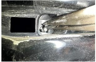
18. Use a pair of needle nose pliers to twist off and remove the three metal ears on each of the two driver side rivets. Next, use a punch to push the center of each rivet through the mounting holes in the rear fascia to remove the rivets.
