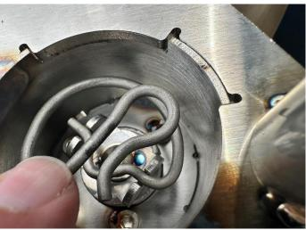
Locate the actuator engagement spring from the passenger FACTORY VALVE ACTUATOR. Position the actuator spring onto the top of the valve as shown.
