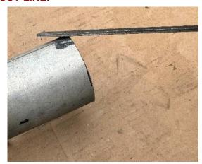
**29.** Thoroughly deburr both cut edges of the **FACTORY TUNNEL** exhaust section.
