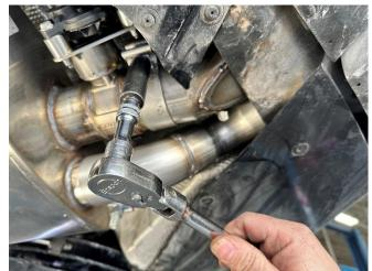
**46.** Secure the passenger inner tip pipe using a ratchet and 15mm deep socket, until the inner tip pipe inlet is snug on the muffler outlet. Leave the clamp connection loose enough for adjustment.
