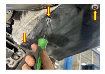
**30.** (ADDITIONAL STEP FOR CT5-V Non-Blackwing ONLY with OPTIONAL FACTORY BEZEL TIP REMOVAL) Locate the six screws set aside in REMOVAL STEP 14. Reinstall the 6 screws (3 per side) securing the side under paneling to the exhaust heat shielding using a T15 Torx Screwdriver.
