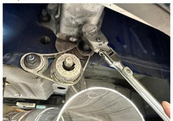
16. Locate two of the nuts set aside in REMOVAL STEPS 12 (CT4/5-V BW ONLY) or REMOVAL STEP 21 (CT5-V NON-BW ONLY). Slide the passenger rear hanger grommet onto the studs in the chassis as shown. Secure the grommet to the chassis using a 3/8" drive ratchet and 15mm socket.
