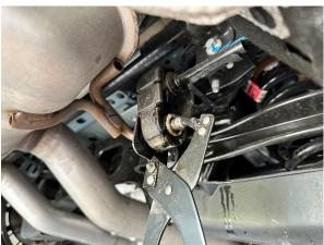
9. Remove the driver and passenger side front muffler hangers (located behind the rear suspension) from the factory grommets using grommet pullers or a similar device.
