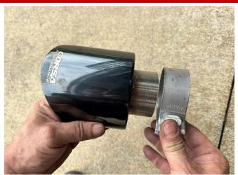
27. Locate a 3.0" clamp and one of the CORSA stainless (or Carbon) outer tip assemblies. Slide the clamp over the tip inlet, so that the nut will be located on the outside top of the tip inlet and facing diagonally downwards. Slide the outer tip assembly onto the passenger outer tip pipe with approximately 1.75" of overlap.
