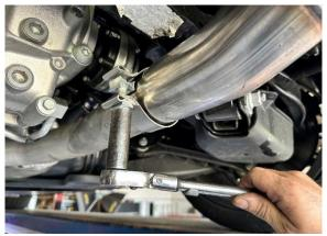
9. Secure the passenger muffler using a ratchet and 15mm deep socket, until the muffler inlet pipe is snug on the axle pipe outlet. Leave the clamp connection loose enough for adjustment.
