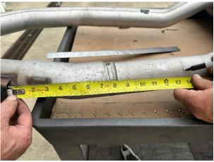
27. Measure 13.5" rearwards (towards the factory muffler) from the rearward edge of the driver side axle pipe hanger bracket as shown, following the outside profile of the exhaust pipe, to mark the CUT LINE.
