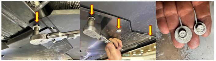
3. To access the center Cross Member, remove the 8 bolts (4 per side) securing the plastic underside panels over the ends of the Cross Member with a 3/8" drive ratchet and 10mm socket. Note the two inner bolts have a large integrated washer, and the remaining 6 outer bolts have a small integrated washer.
