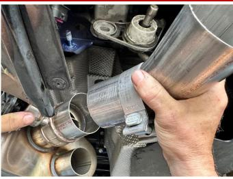
**15.** Slide the passenger inner tip pipe assembly onto the passenger muffler outlet, with a recommended pipe overlap of 1.625 inches.
