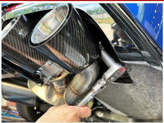
28. Adjust the rotation of the CORSA outer tip assembly until the CORSA logo is centered on the top of the tip, then secure the exhaust clamp at the tip inlet using a 15mm socket and 3/8" ratchet, until the tip is snug on the outer tip pipe. Leave the clamp connection loose enough for adjustment.
