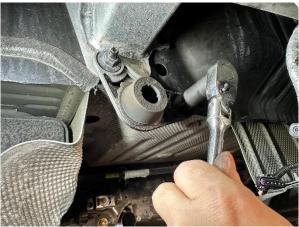
21. Use a 3/8" drive ratchet and 15mm socket to remove both nuts securing each of the driver and passenger side rear hanger grommet assemblies. Set aside the fasteners in a protected location to be reused during INSTALL STEP 16.
