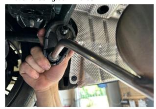
8. Slide the front muffler hanger into the corresponding grommet as shown. Rotate the passenger muffler until the hanger is horizontal as it runs through the stock grommet.
