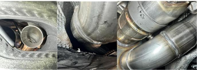
**49.** Adjust the passenger outer tip pipe rotation and position until the pipe is centered within the factory bezel tip, and the pipe has clearance to both the outer exhaust heat shielding and the passenger inner tip pipe as shown.
