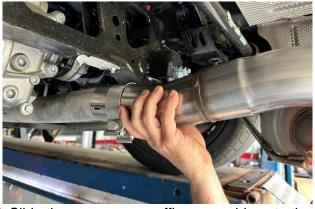
**33.** Slide the passenger muffler assembly onto the passenger axle pipe outlet (or passenger outlet of the **FACTORY TUNNEL** section), with a recommended pipe overlap of 1.75 inches.
