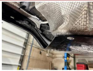
**24.** The edge of the cut should make a clean transition to the edge of the tip cutout in the rear fascia and should align with the exhaust heat shielding as shown.
